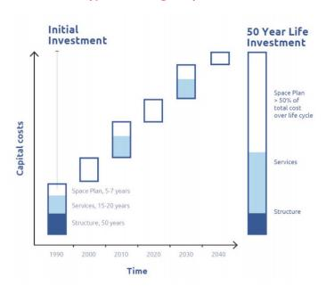
As this diagram demonstrates, the cost of space plans – how you organise the layout of a building - and services are much higher than the cost of the structure over a building's life.
